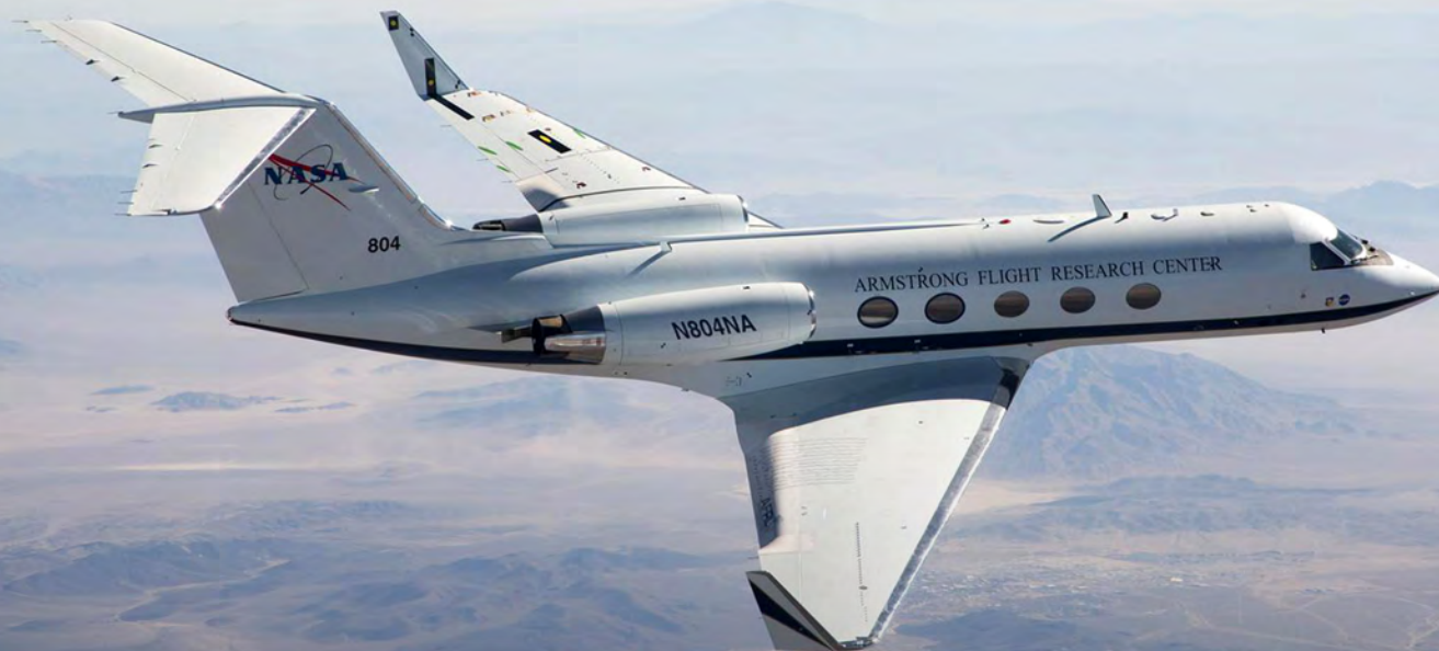
In 2015 trials for NASA and the U.S. Air Force Research Laboratory, FlexSys flew this modified Gulfstream II with a morphing flap that spanned the middle portion of one of the wings.
