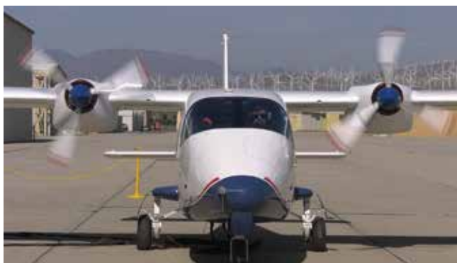
▲ The electric motors for NASA's X-57 Mod II vehicle and their propellers are powered up and spun for a test. The X-57 Maxwell is an Italian Tecnam P2006T aircraft NASA is modifying to fly electric in three configurations to lay the groundwork for certification standards for future electric aircraft. The Mod II is the first of the configurations.
