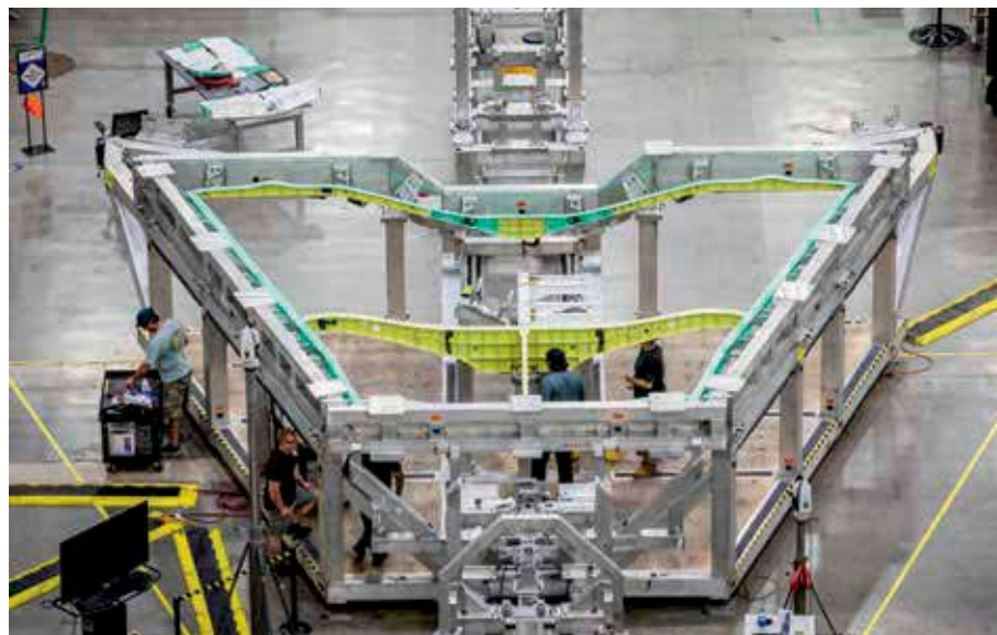
▲ NASA's X-59 Quiet Supersonic Technology airplane, including parts of its wing, is under construction at the Lockheed Martin Skunk Works factory in Palmdale, California. The yellow and green parts at the top are the aft-wing structure; in the center is the mid-wing structure. The silver is tooling. Lockheed Martin
