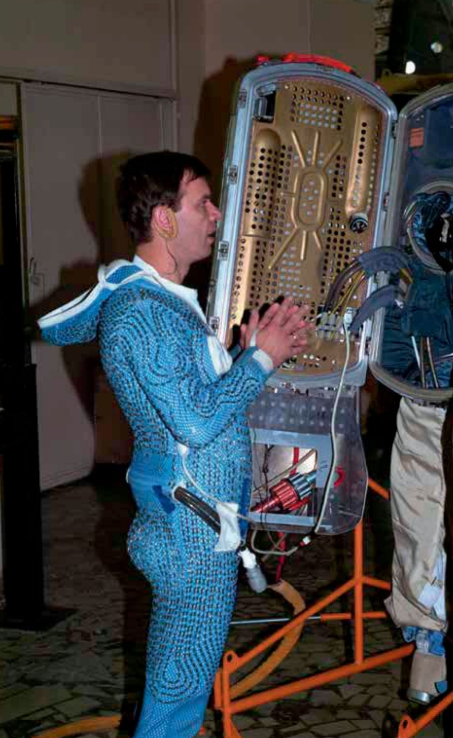
▲ Cosmonaut Yuri Gidzenko wears a thermal undergarment as he is about to put on an Orlan space suit at a test center in Russia. A similar rear-entry hatch will be incorporated into NASA's xEMU. NASA
