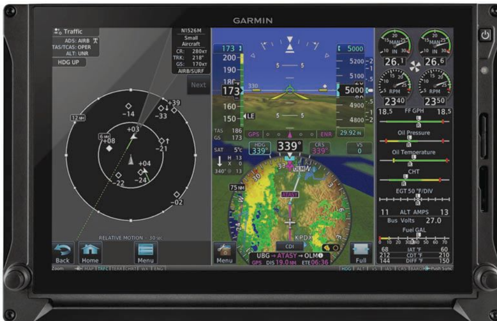
◀ ADS-B air traffic is indicated by white diamonds on the left side of this cockpit screen. A receiver picks up the signals and relays them to the G600 TXi display, which can be installed on single- and twin-engine general aviation aircraft.
