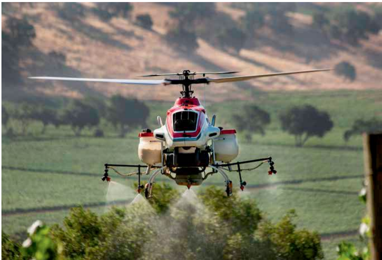
▲ Yamaha's RMAX remotely piloted helicopter is the largest unmanned aerial application aircraft flying in the U.S.
