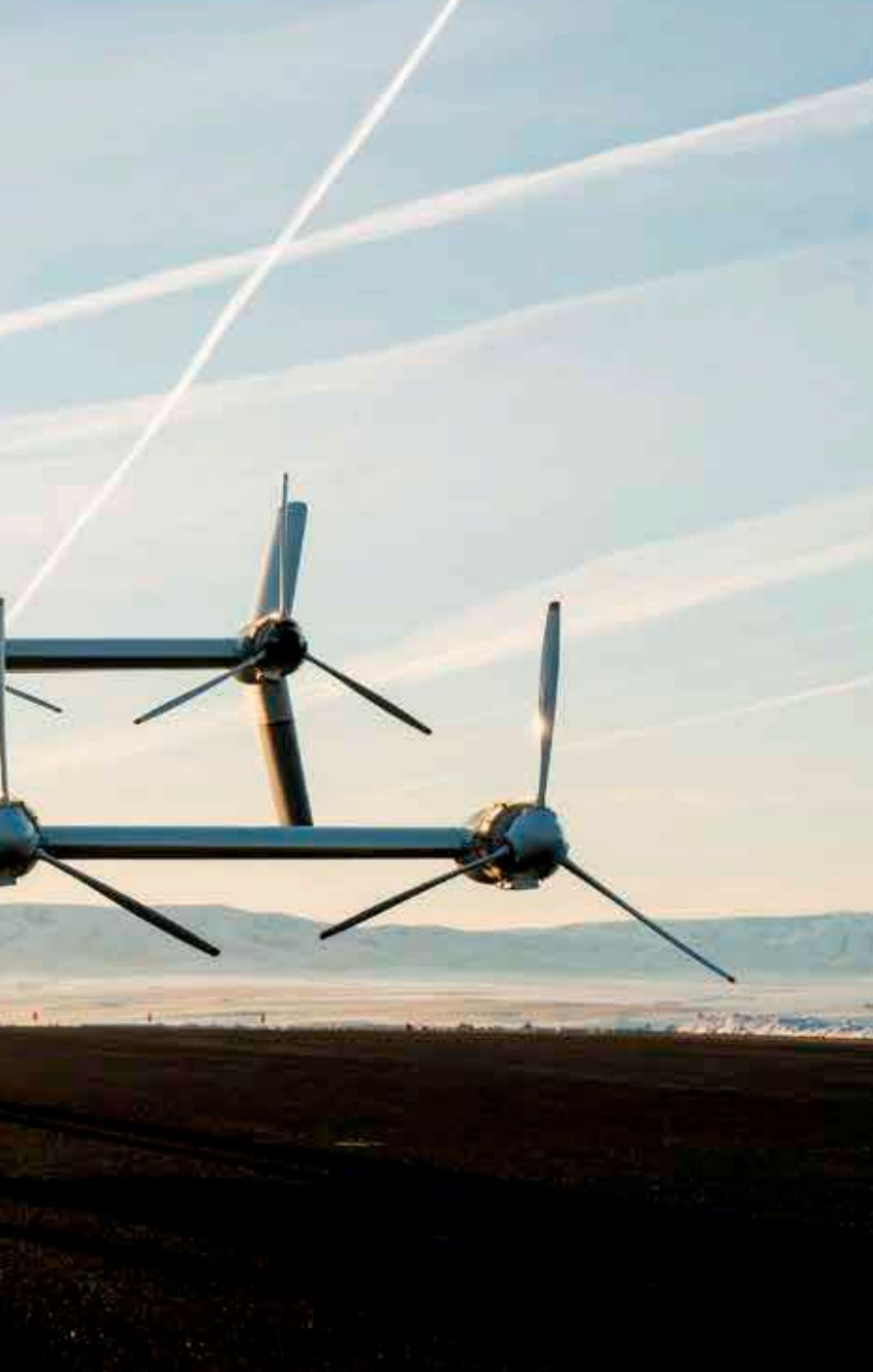
▲ Vahana, an all-electric, self-piloted urban air mobility demonstrator. Airbus
