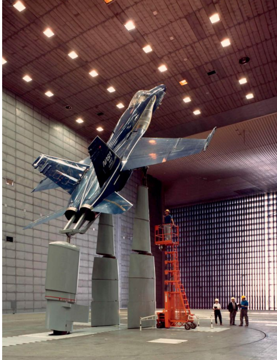
▲ An F/A-18 fighter aircraft is tested for high angle-of-attack aerodynamics in the 80-by-120-foot wind tunnel at NASA's Ames Research Center in California.
