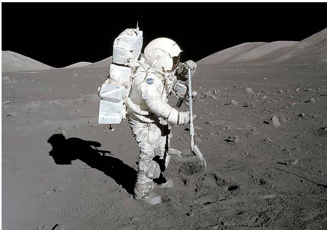
◀ Apollo 17 astronauts Gene Cernan and Jack Schmitt collected 110.5 kilograms of lunar regolith during their three spacewalks. In this photo taken by Cernan, Schmitt drags a rake through lunar soil and shakes it to dislodge small rocks.
