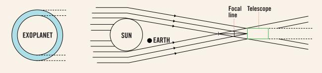
Sources: Louis D. Friedman and Slava G. Turyshev Diagram is not to scale The smallsat will have months and years to observe the target exoplanet, deconvolute the image, and communicate to Earth -a virtual orbiter of the distant exoplanet.
