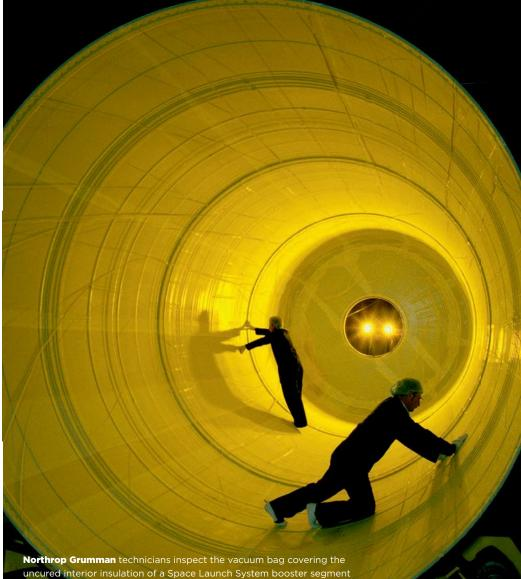
Northrop Grumman technicians inspect the vacuum bag covering the uncured interior insulation of a Space Launch System booster segment prior to autoclave curing. A good vacuum bag seal is critical for holding the uncured insulation in place and for gas removal during the curing process.
