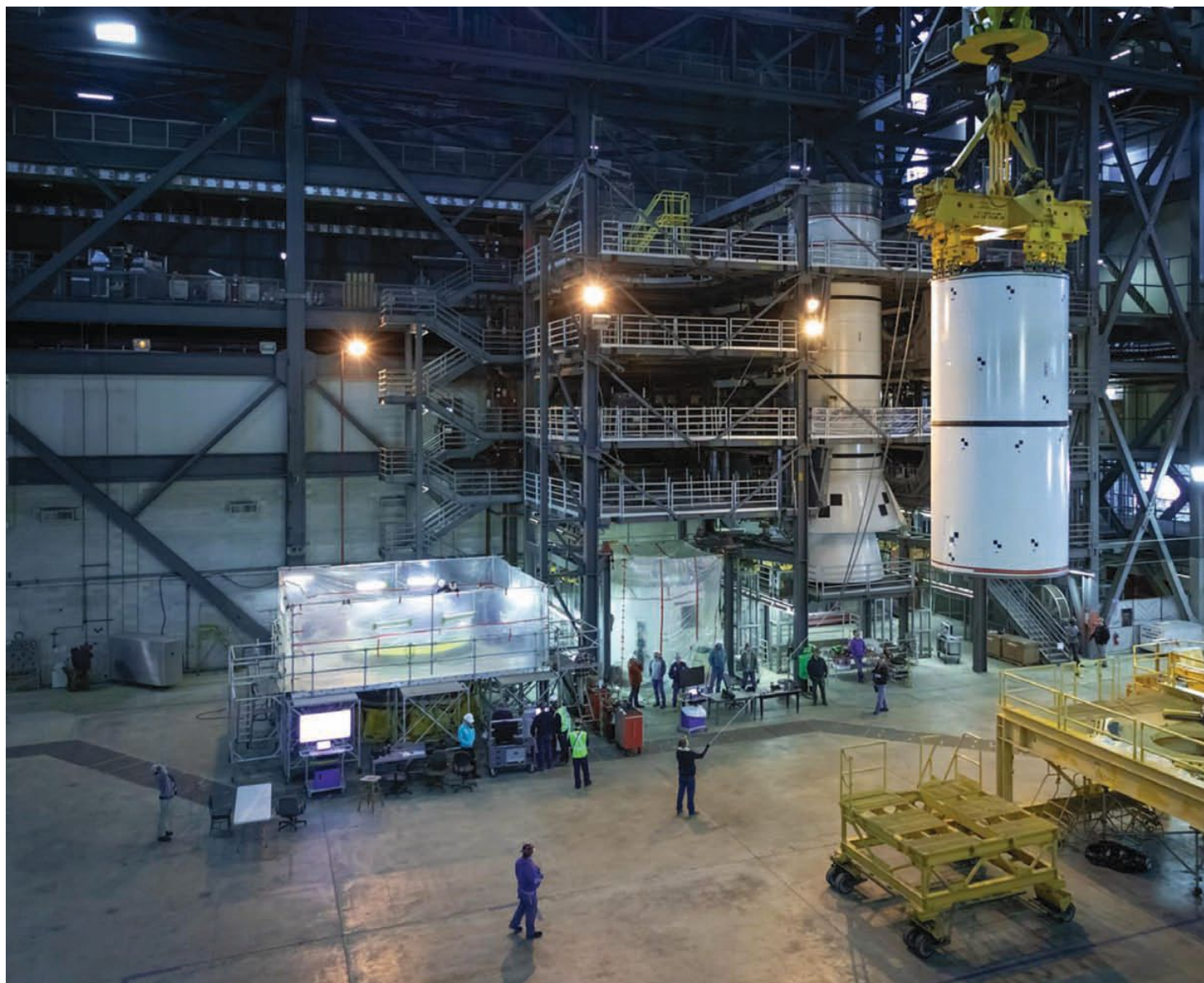
▲ Engineers, technicians and crane operators practice moving Space Launch System solid rocket booster test segments at NASA's Kennedy Space Center in Florida.
