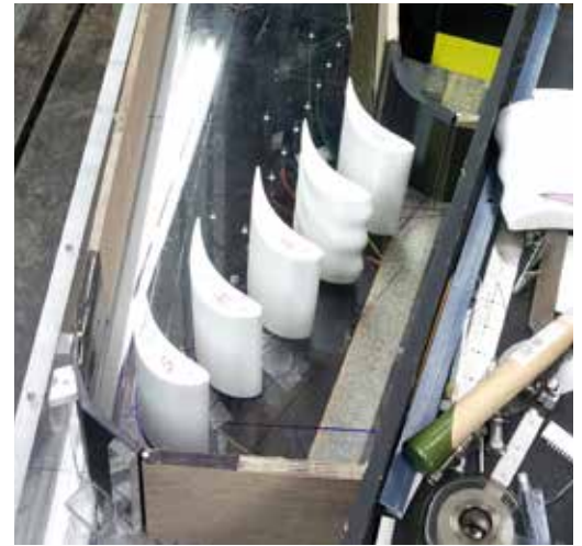
▲ A wavy blade design based on a harbor seal whisker was tested among reference blades in a transonic wind tunnel at NASA's Glenn Research Center. Test blades are geometrically larger than real turbine blades to better characterize the flow physics.
