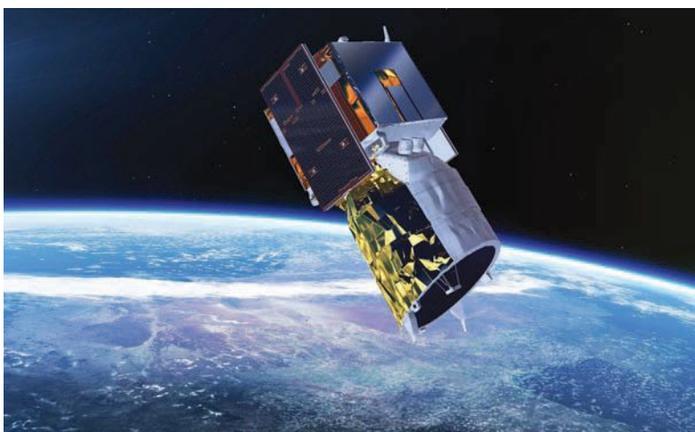
▼ An illustration of the Aladin instrument, a wind lidar, aboard the Aeolus satellite.
