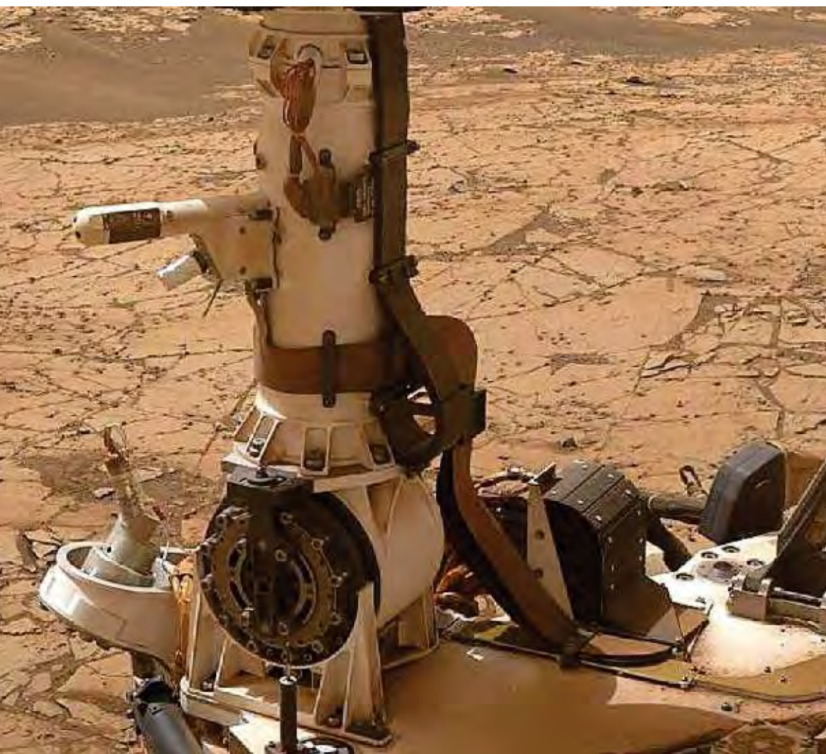
This image taken by the Curiosity rover on the Martian surface shows the extended length flex flight part (brown, flat cable that starts on deck and wraps around the mast) that powers the camera and the rest of the rover.
