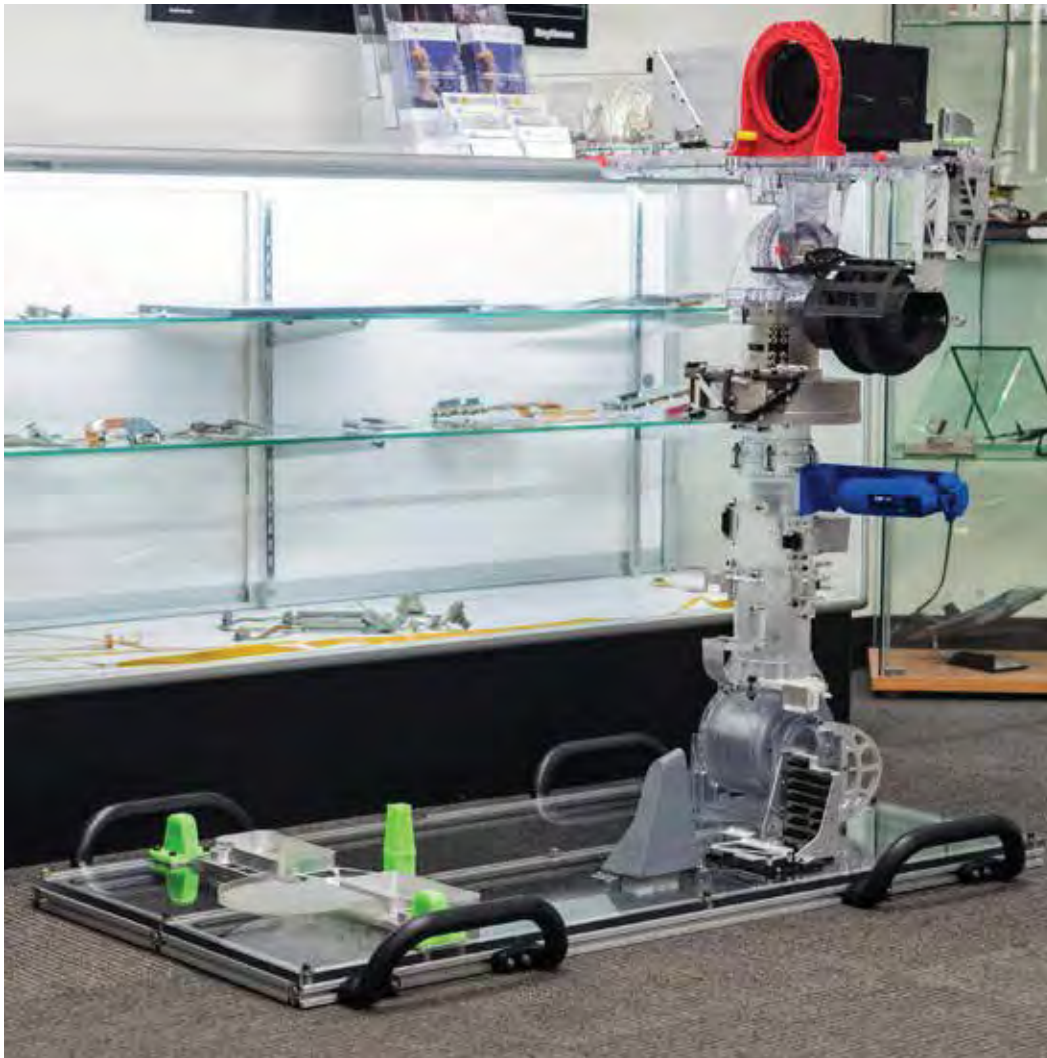
▲ Pioneer Circuits tested its latest flexible circuitry on this mock-up of the Mars 2020 rover's mast. NASA
