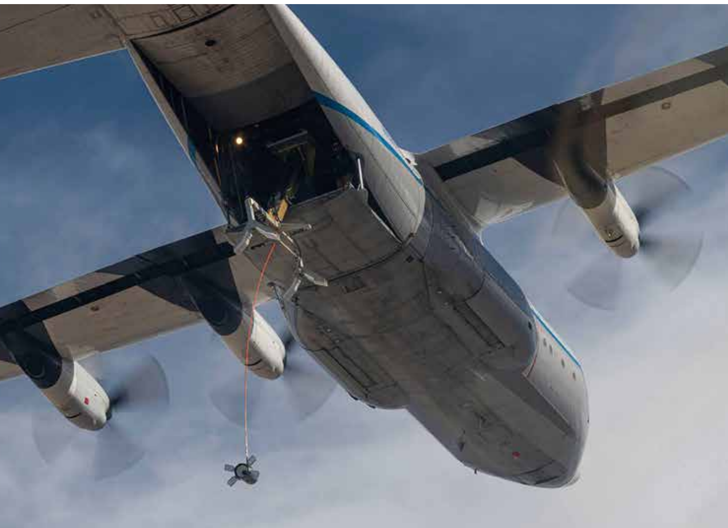
▲ A Gremlin drone approaches a C-130A cargo aircraft over the desert near Dugway Proving Ground in Utah. The recovery of this particular Gremlin was the culmination of nearly two years of test flights.
